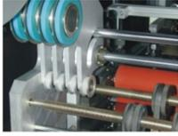
Double adhesive tape tracks with tape guiding rollers for tape width from 2mm to 10mm.
