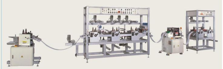
The Chinup HSM-03 is specially designed for small cut parts. Short cutting stroke and feed distance shorten the cutting cycle substantially and lead to much higher output. Flexible production stations are available to meet different demand of variable job application.
