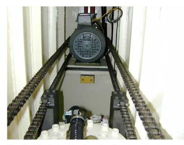
The double chain drive traveling head mechanism ensures the smooth traverse movement of the head. Therefore durability of the related machine parts is greatly increased.
