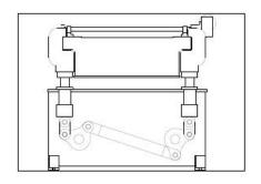
two-speed cutting stroke that provides maximum speed on the down stroke and accurate control of the cutting position to optimize production rates while extending die and pad life.
