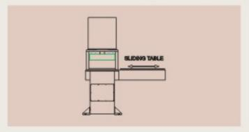
☐ Single auto hardened & ground steel sliding table (kiss cutting & through cutting).
