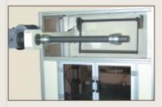
Scrap rewind device. Cutparts and waste web separating device and cutparts rewind stand can be equipped for kiss cutting job.
