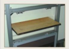
Side loading pneumatic die rails for easy die loading.
