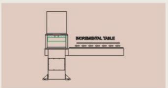
Servo-drive incremental hardened & ground steel sliding table feeding system (kiss cutting & through cutting). Table length according to sheet type material length.
