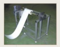
Air shaft core clamp motorized single roll material stand with lazy loop control to minimum material tension during feeding. There is simple one roll material stand available without air shaft and lazy loop control.
