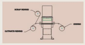
Servo-drive inboard & outboard pinch roll feed with cutparts rewind stand (kiss cutting) and overhead scrap rewind stand (kiss cutting & through cutting).
