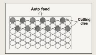
□This cutting die layout with material auto feed can achieve much more yielding output than conventional cutting method and lead to good material saving.
